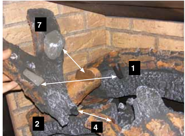
13) Locate provision on the bottom of Log 7 (see highlighted areas), place on provision on Log 1 and in provisions on Log 2 and Log 4 (see darkened areas).
